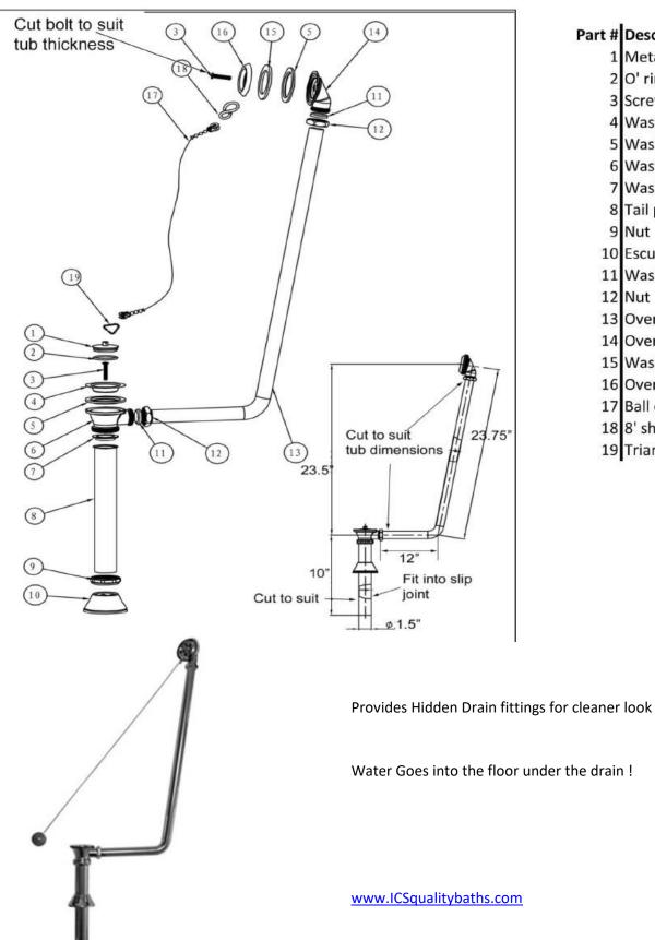
Part # Description 1 Metal stopper 2 O' ring 3 Screw 4 Waste Flange 5 Washer 6 Waste body 7 Washer 8 Tail pipe 9 Nut 10 Escutcheon 11 Washer 12 Nut 13 Overflow pipe 14 Overflow body 15 Washer 16 Overflow flange 17 Ball chain 18 8' shape connector 19 Triangle connector
